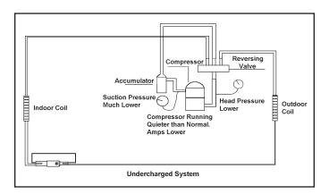
it is an indication of a low refrigerant charge. A check of the amperage drawn by the compressor motor should show a lower reading. (Check the Unit Specification.) After the unit has run 10 to 15 minutes, check the gauge pressures.
